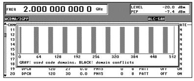
The code channels are equally distributed over the code domain. The influence of TOFFS = 0 for all code channels cannot be seen from this display
