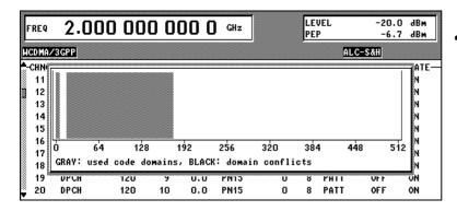
As the channelization codes are assigned in ascending order the code channels are not equally distributed over the code domain
